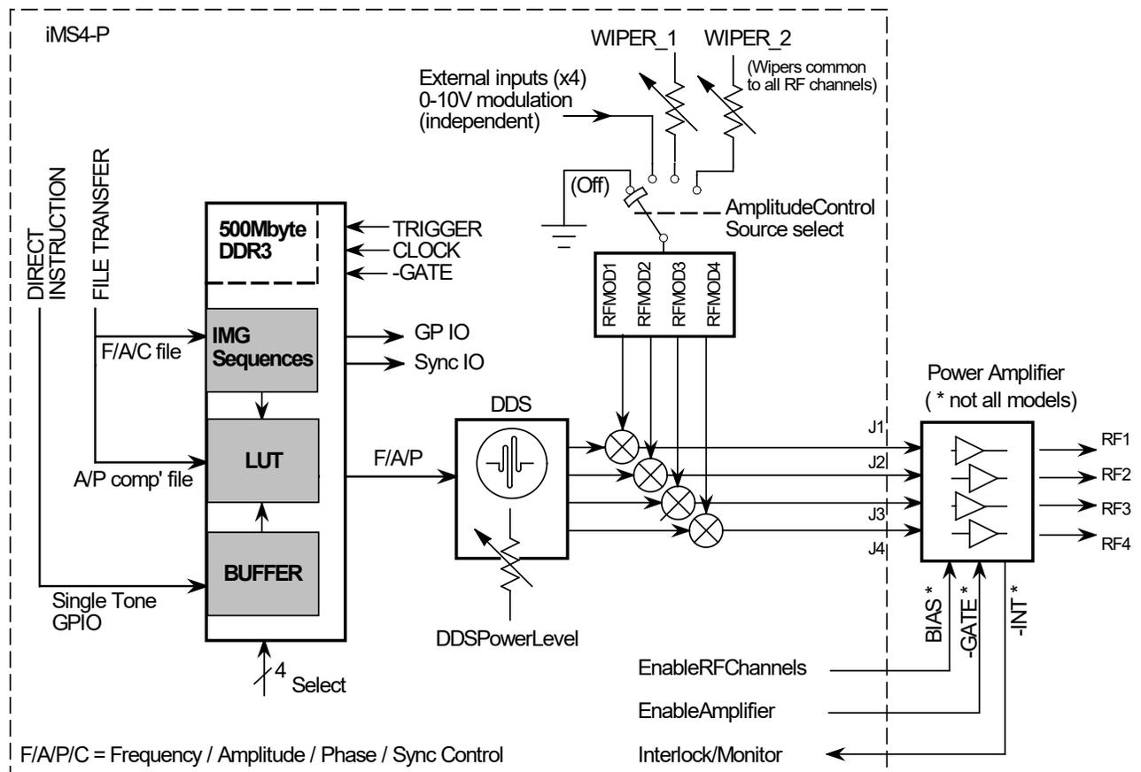
The iMS4 synthesizer operates in three basic modes
