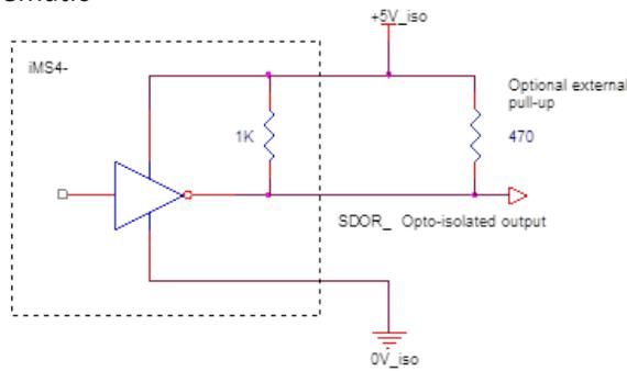
Diagram shown with optional external pull-up resistor to improve the rising edge. Min value 330ohm
