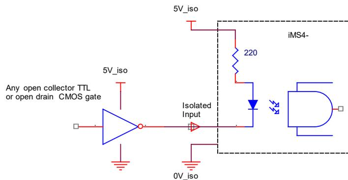
Opto-isolated logic output schematic
