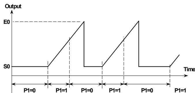
A **Frequency Sweep Dwell** only returns to the start value after a falling edge transition on the appropriate profile input
