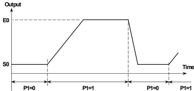
Both plots show a ramp on output J2, controlled using input P1
